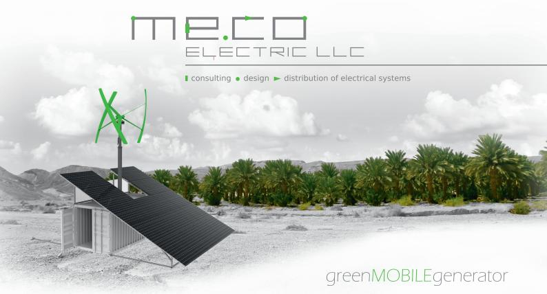
The greenMOBILEgenerator is a standalone hybrid power system for electrification of areas which are not reached by the grid. It is a compact and modular unit, using solar and wind energy to delivery uninterrupted clean energy. The containerized system has a peak power output of 10 kWp and an average power output of 40 kWh per day in standard version. The output can easily be increased up to 30 kWp by adding additional ground-mounted solar panels.
